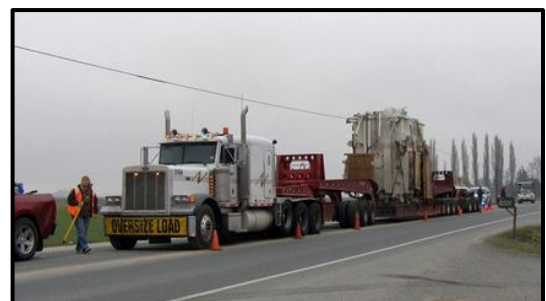
Super-load requiring bridge loading analysis.
